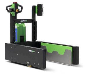
Power: Max pull: Speed: Battery: Working height: Motor 24V, 700W Up to 1500kg 4,5 km/h Repleceable lithium 24V 800 - 1100 mm
