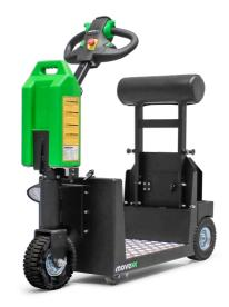
Power: Max pull: Speed: Battery: Working height: Motor 24V, 420W Up to 1000kg 6,5 km/h Repleceable lithium 24V 1082 - 1223 mm
